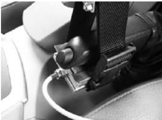
Fig 2: Sensor type CPFTB... mounted at the hand brake lever of a car
