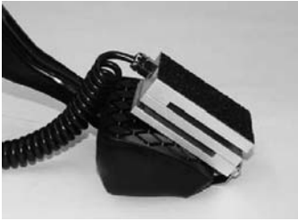
Fig 1: Sensor type CPFTB... mounted at the brake pedal
