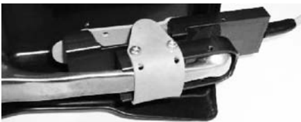
Fig 3: Sensor type CPFTC... mounted at the hand brake lever of a motorbike
