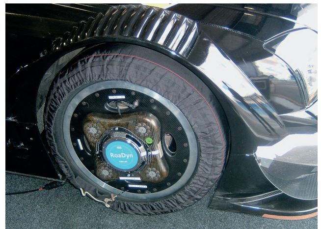
Fig. 2: Race car with RoaDyn® S625 System 2000
