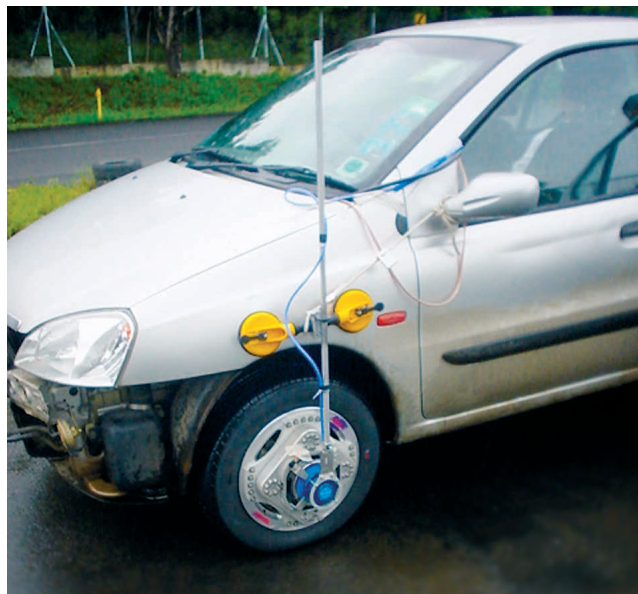
Fig. 4: RoaDyn® S625 made of aluminium with out-board transmission for small rims
