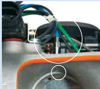
Piezoresistive absolute pressure sensor Type 4005B... mounted in the inlet manifold
