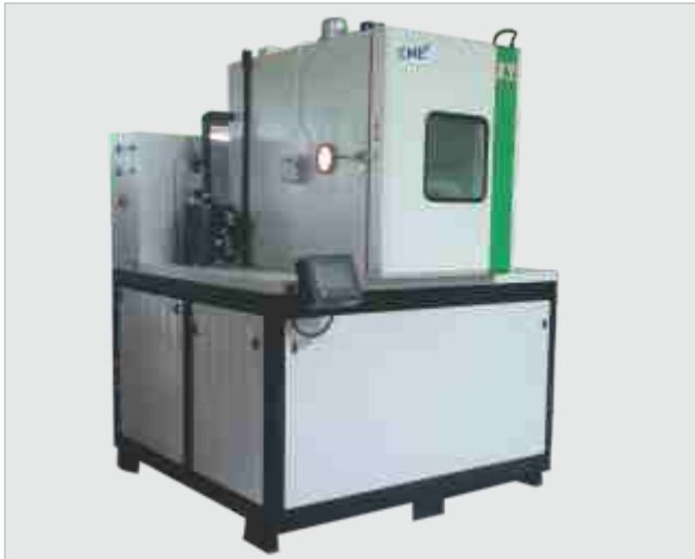
ESS High ramp rate Chamber 20 deg / min
