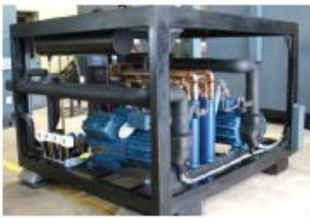
Remote Refrigeration: Refrigeration units can be placed away from the main chamber and are mounted on heavy duty chassis.
