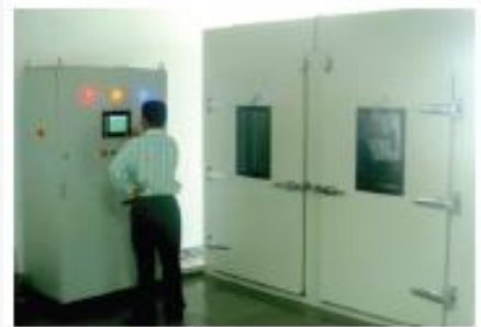
Remote Control Panels: The control panel housing the electrical switchgear and the operating interface enviCoM are available as independent stand alone units. These units can also be placed at a remote location.
