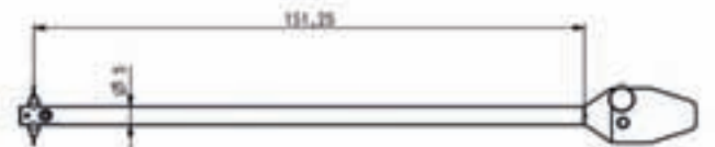
Probe arm with double probe tip from 16 mm Probe arm length 200 mm Probe ball radius 250 μm
