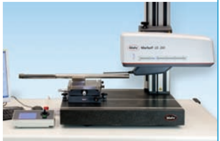
Rack measurement with MarSurf LD 260
