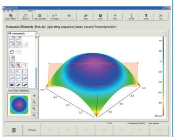
In the case of molds for items such as contact lenses, the surface topography is also of interest in addition to the individual profile for determining the roughness depth.
