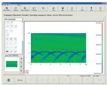
Different machining methods produce different surface structures. The machining structures are often very disparate which means that one single tactile profile cannot provide representative information about the profile character.
