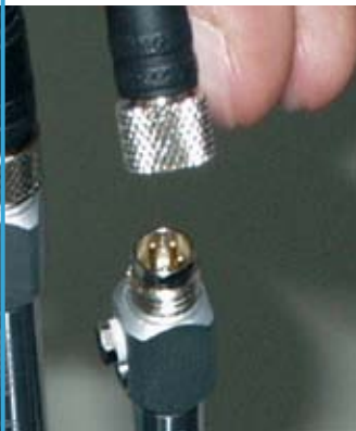
Cable and probe can be separated with the plug-in connector.
