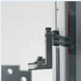
Probe contact with the motorized measuring carriage.
